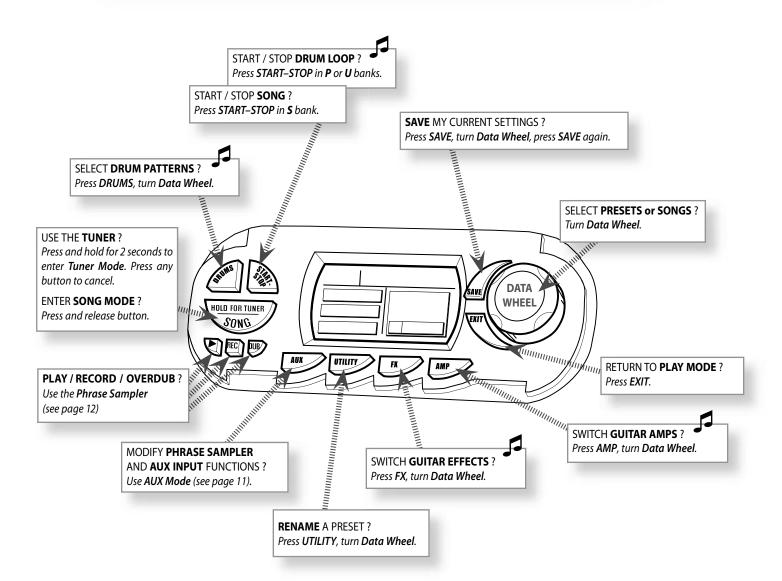
Shortcuts—Press and hold this button while rotating the Data Wheel to make a quick adjustment without leaving Play Mode (except in "S" bank)
