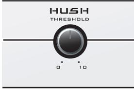
The front panel *HUSH Threshold* control determines the minimum input level at which the HUSH filter and downward expander will begin to operate. Setting this control too high will result in a loss of sustain, as notes will tend to die out much faster than they should. Conversely, when set too low, the expander will close too late (if at all) and the noise floor will remain audible
