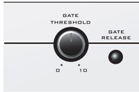
This circuit is combined with the Variable Integrated Release (V.I.R.) circuit to provide an internal variable release to the downward expander. With the V.I.R. circuit, if the guitar signal decays slowly, the downward expander will engage slowly. If the guitar signal stops quickly, the downward expander will engage quickly. The LED indicates when downward expansion is active.
