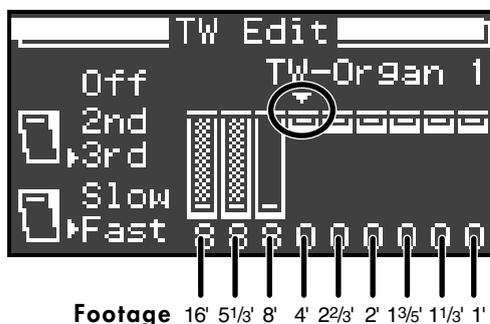
If the TW Edit (tone wheel edit) screen is displayed, you can use the Tone buttons, [Registration] button, and [Split] button to select the desired footage. After selecting a footage, you can also use the [-] [+] buttons to adjust its volume.
