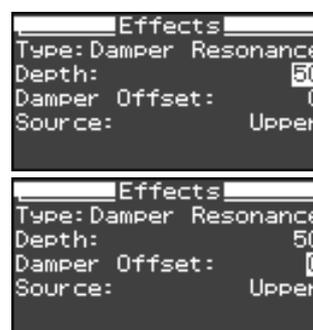
The item in the second line from the top of the Effects screen can be changed by holding down the [Multi Effects] button and using the [-] [+] buttons, without your having to open this screen.
