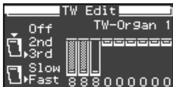
4. Hold down the [Display] button and press the [-] [+] buttons several times to select the footage for which you want to change the volume.
