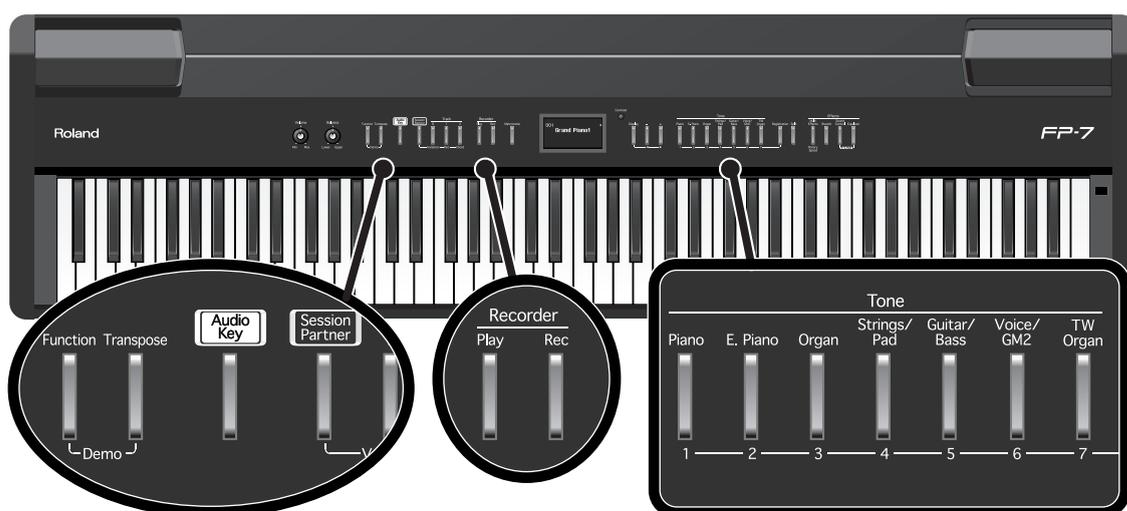
**1. Hold down the [Function] button and press the [Transpose] button.**
