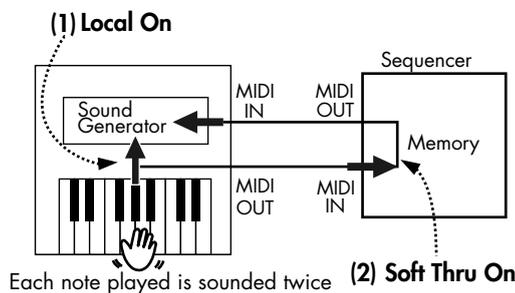
**Local On:** The keyboard and recorder are connected to the internal sound generator.
