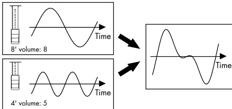
You can simulate the creation of tones using the harmonic bars by assigning footages to the Tone buttons.
