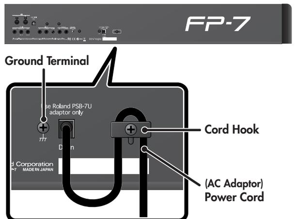
To prevent the inadvertent disruption of power to your unit (should the plug be pulled out accidentally), and to avoid applying undue stress to the AC adaptor jack, anchor the power cord using the cord hook, as shown in the illustration.
