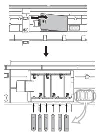
For battery operation the instrument requires six 1.5V "AA" size, LR6 or equivalent batteries. (Alkaline batteries are recommended.) When battery power becomes too low for proper operation, make sure to replace all batteries, following the precautions listed below. If necessary, also make sure to save all important User data (see pages 50, 88).
