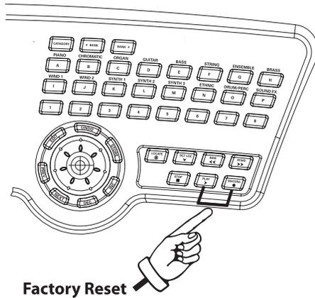
The Fusion has a “factory reset” option that will reset your global parameters to their initial factory settings. This has been included as a last resort option in case you have accidentally changed a global setting and need to return the workstation back to normal quickly.
