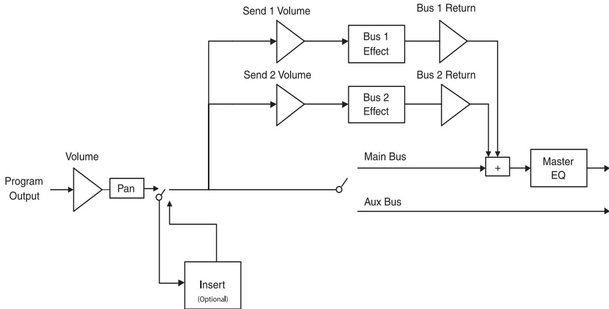
This block diagram describes the flow of the signal after it leaves your Program. The triangles represent volume control points (engineers often use triangles in block diagrams to represent amplifiers).
