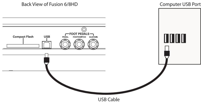
**USB:** Connect your Fusion to a Mac or PC for easy file transfers. The Fusion supports USB 2.0 and is fully backwards-compatible with USB 1.1/1.0, but we highly recommend using 2.0 since audio files tend to be quite large and transfers will be slower on USB 1.1/1.0 connections.
