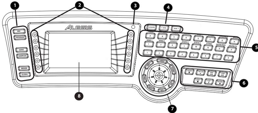
**1. Mode Selection Buttons** (Mix, Program, Song, Sampler, Mixer and Global): These buttons select the main modes of the Fusion.
