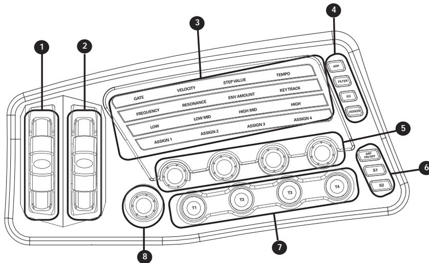
The Fusion’s Performance Panel has several real-time controllers (wheels, knobs, buttons, and switches) that you can assign to perform a variety of tasks. These controllers let you tweak sounds in real-time as you play for maximum expression and sonic control.
