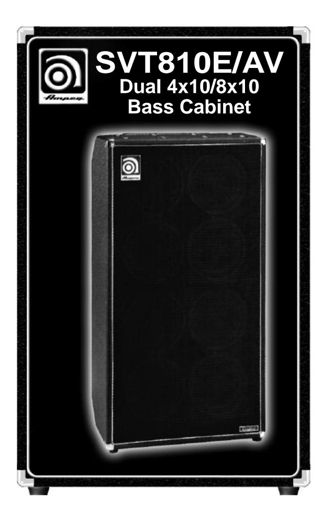
Your Ampeg SVT-810E/AV Dual Bass Cabinet is a high quality speaker cabinet suitable for all sizes of venues. The SVT-810E/AV can be "split" into two isolated 8 ohm, 4x10 cabinets via the jackplate connections. This allows each cabinet to be driven by a separate amplifier. Of course it may also be connected in the Mono Mode to create a single 4 ohm, 8x10 cabinet that may be powered by a single amplifier.
