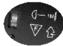
AC Voltage Switch Example
