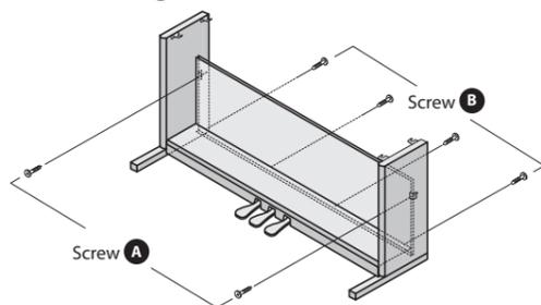
**7.** Go around and tighten all the screws, while at the same time correcting the orientation of any piece that needs it, until everything fits together properly.
