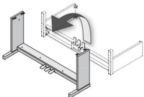
**4.** Place the rear board as shown below and adjust the screw holes of the rear board and the pedal board.
