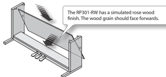
**5.** Attach the rear board to the metal parts on the side boards from the front using screws A (4 x 14 mm).
