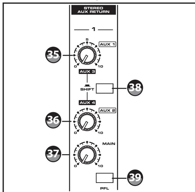
The L Series feature two additional STEREO AUX RETURN inputs that can be used to return the outputs of the an external effects processor, or to connect the output of any stereo line level device. The STEREO AUX RETURN can be routed to the MAIN mix, or to a pair of AUX outputs, allowing you to send the signal to a monitor mix.
