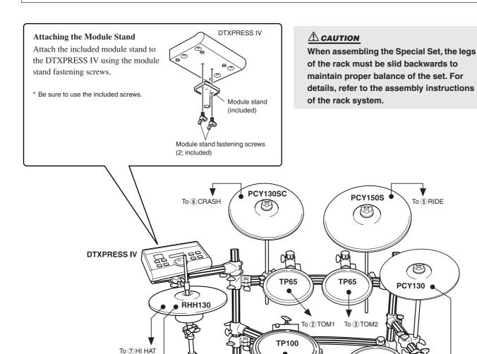
\* First, connect the RHH130's [PAD] output jack to the 7 HI HAT jack on the DTXPRESS IV, then connect the RHH130's [HI HAT CONTROL] output jack to the HI HAT CONTROL jack on the DTXPRESS IV.
