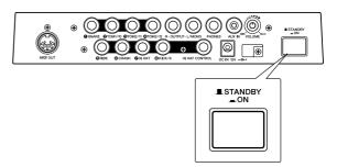
**4-3.** To turn off the power, press the [STANDBY/ON] switch again.
