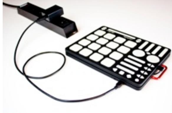
The red charging LED indicator will not turn on if Rogue is already fully charged. Charging will cease when the battery is full. This means that if you leave the Rogue on while charging, it might charge fully and then wear out again – it will not charge back up unless it is unplugged and then plugged back in.
