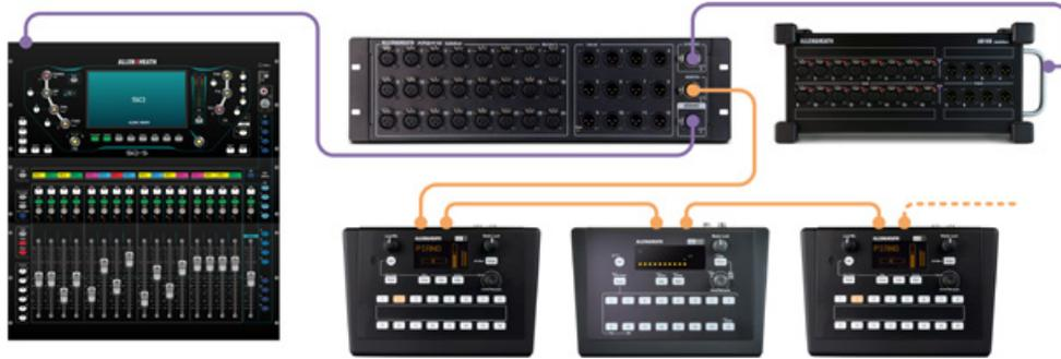
SQ expanded with 2 x DX168 for full 96kHz operation
