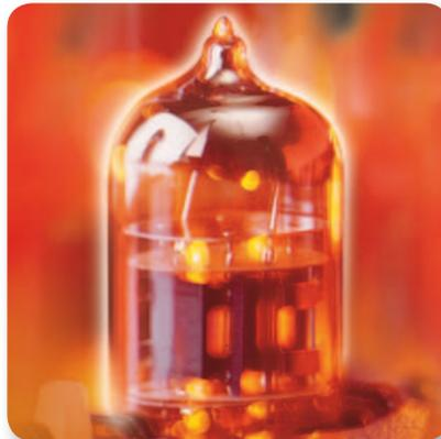
Often employed in British-style amplifiers, the EL84 output tube is known for its crisp and chiming tonal quality when pushed to the max, and the V22HD harnesses every ounce of that power to awesome effect.
