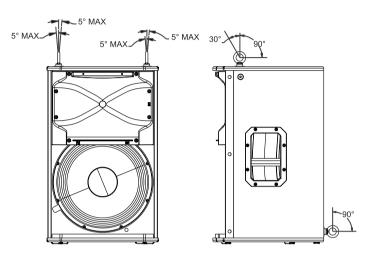
Figure 5.4: Maximum working load - vertical orientation
