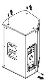
2. Replace the **M10 screw** with the fender washer and eyebolts.
