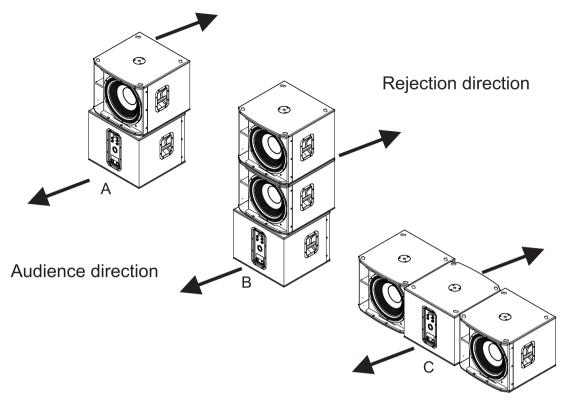
Figure 7.2: Cardioid physical alignment
