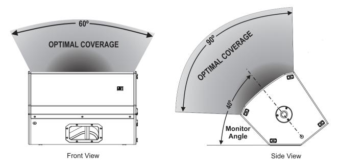
Figure 4.3: Optimum coverage in monitor position
