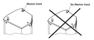
Figure 5.2: Eyebolt shown with and without washer
