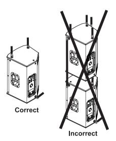
Figure 5.5: Loudspeaker vertical suspension
