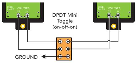
Solder points located on rear of pickups
