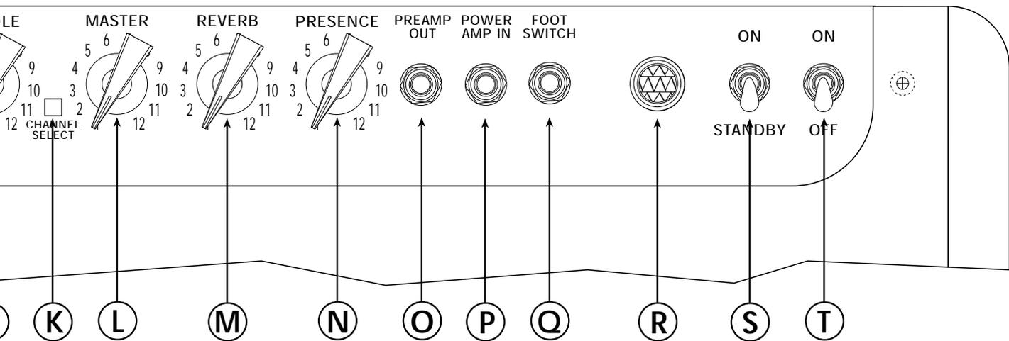
**K. CHANNEL SELECT** - When this button is pressed, the amp switches from the NORMAL channel to the DRIVE channel.
