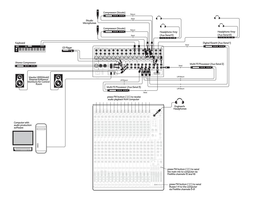
This diagram shows studio mics connected to the channel 3 and 4 mic inputs and a keyboard connected to the channel 6 and 7 line inputs. This allows for overdubs when necessary. A CD player connects to the tape input for referencing pre-recorded material.
