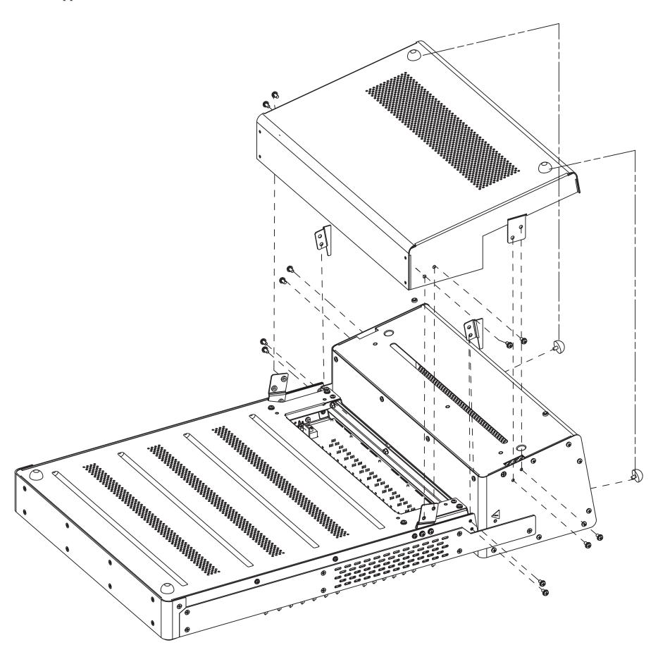
This step is optional. Remove the 14 screws from the two side trim pieces. Screw the rack ears to the mixer where the side trim pieces used to reside. You will only use eight screws (four on each side) for the rack ears. The trim pieces and remaining screws should be stored away for safekeeping.
