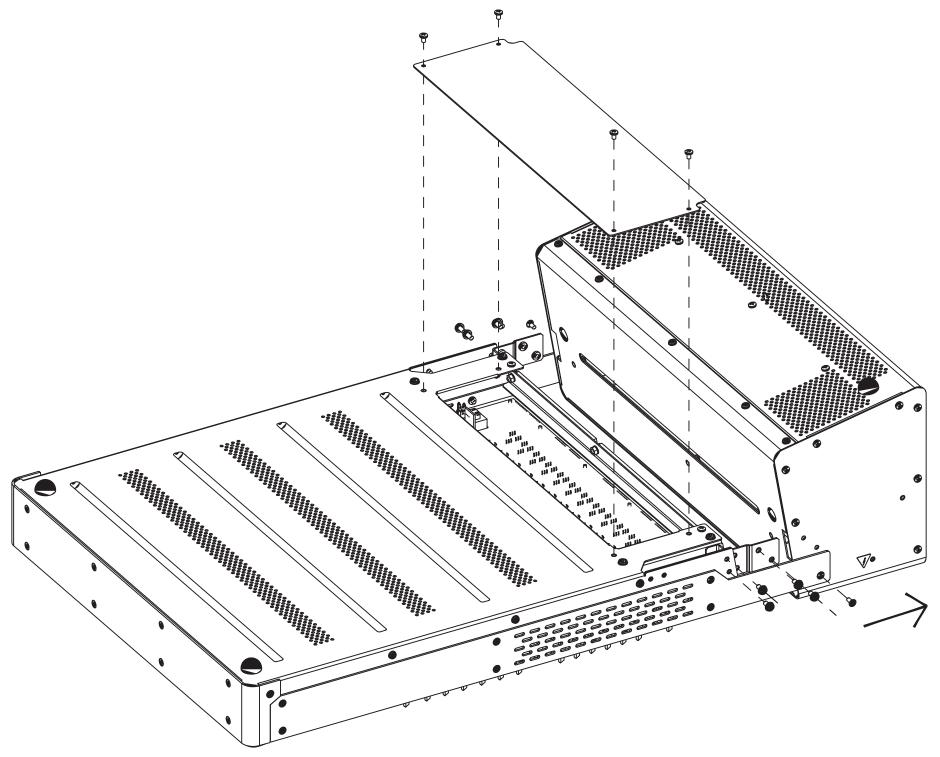
Rotate the Pod arms and reinstall the four arm screws. Rotate the Pod so that the connection jacks are parallel to the top of the mixer. Reinstall the two silver flathead screws through the side trim and back into the Pod.
