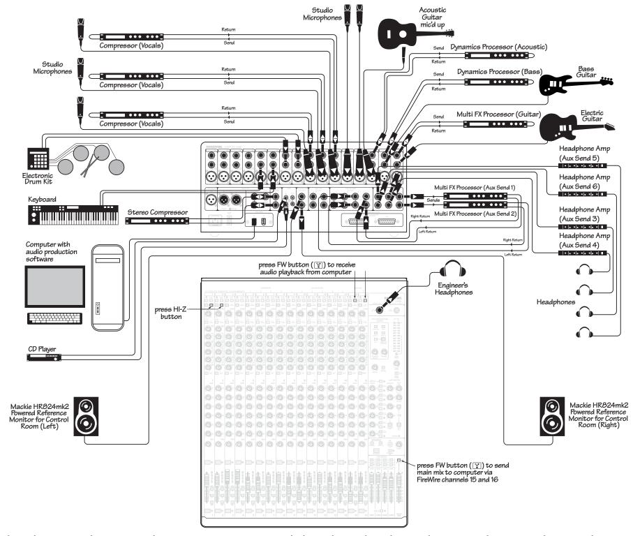
This diagram shows an electric guitar connected directly to the channel 1 input (hi-z switch in), a bass guitar connected directly to channel 2 (hi-z switch in), an acoustic guitar mic connected to the channel 3 mic input, studio mics connected to channel 4-8 mic inputs, an electronic drum set connected to channel 9-10 line inputs, and a keyboard connected to channel 11-12 line inputs. A CD player connects to the tape input for referencing pre-recorded material.
