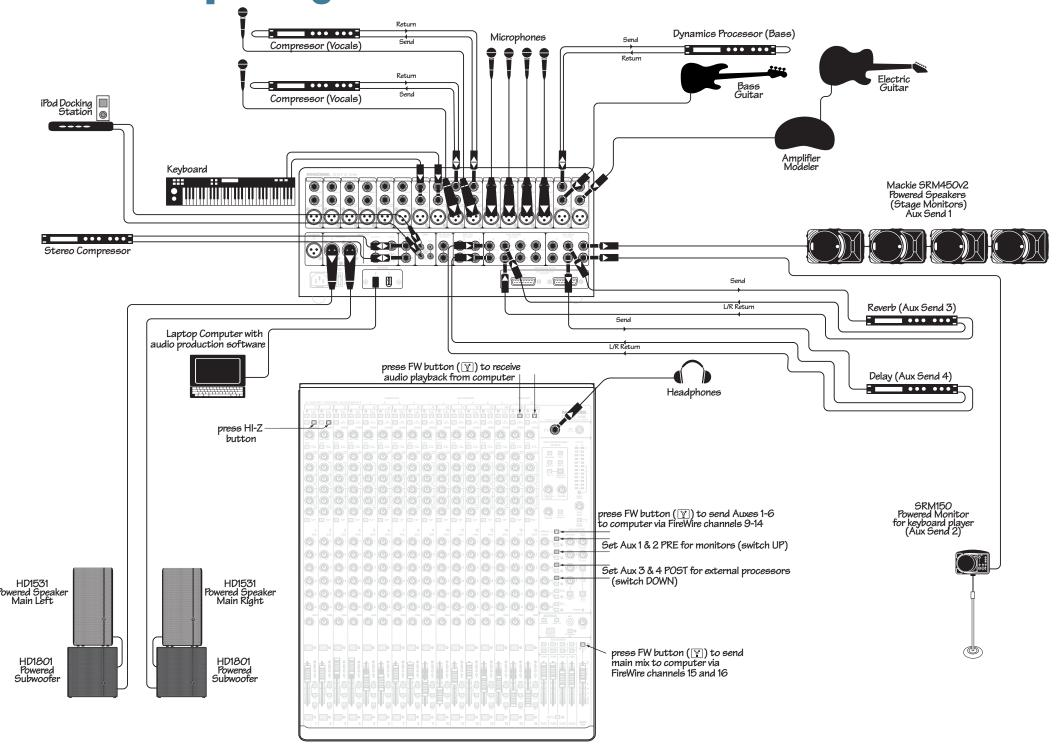
This diagram shows an electric guitar connected to the channel 1 line input via an amp modeler, a bass guitar connected directly to channel 2 (hi-z switch in), microphones connected to channel 3-8 mic inputs, and a keyboard connected to the channel 9 and 10 inputs. An iPod® dock connects to the tape input. Headphones are used to monitor levels.
