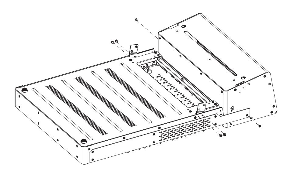
6. Attach the two triangular cosmetic pieces with the supplied screws. Place the Pod bucket as shown. Attach the Pod bucket to the mixer using the screws removed in step 3. Screw the Pod bucket to the Pod using the supplied screws. Unscrew the feet from the Pod and reattach them to the Pod bucket.
