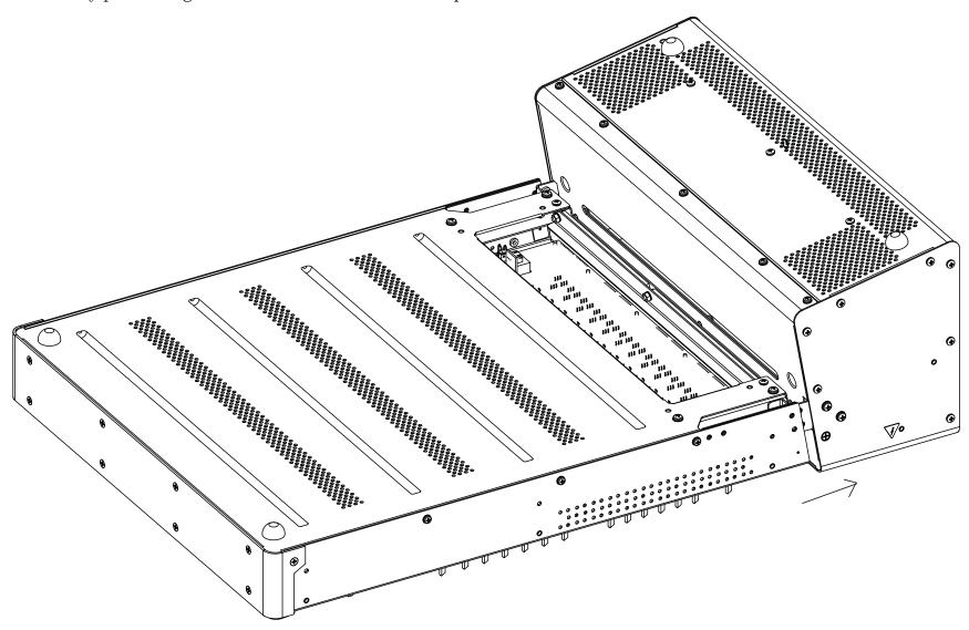
Rotate Pod as shown below. Hold both sides of the Pod to keep the travel even. Move the Pod all the way back until it stops and the bottom surface of the Pod is parallel to the bottom of the main unit.
