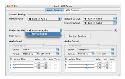
You can also choose it as your default input or output, as well as designate it to be used for system sound output. There are 16 channels of audio input from the Onyx 1640i, and 2 channels of audio output to the Onyx 1640i.
