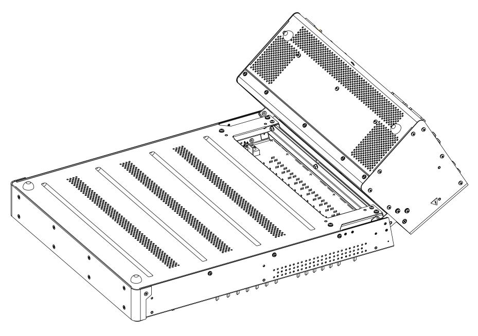
The Pod should drop down on to the chassis after a complete rotation. Give 'er a good wriggle if the screw holes do not line up properly. Reattach the recently rotated Pod with the four screws removed in step 3. Attach the rack ears to the mixer using the same silver flathead screws removed from the side trim. The rack ears are stamped with an 'R' or 'L' to denote which side of the mixer it goes on, based on house view. Finally, attach the wire cover bracket with the screws that it arrived with.
