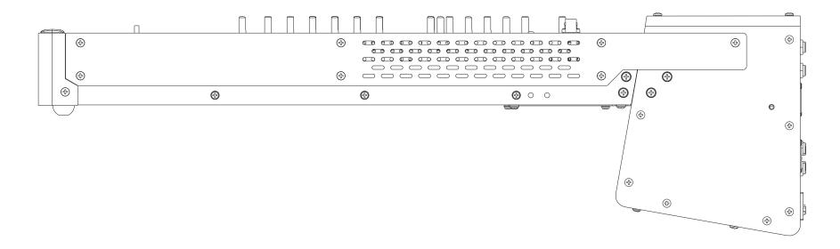
2. The Pod can be fitted on the back of the mixer, with the connections pointing out the back. This will take up 12 rack spaces. (Allow one or two extra spaces for making your connections.) Details follow on how to change to this configuration.
