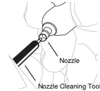
**Warning:** The cleaning tool is only to be used to clean the earphones. Any other use, such as using the tool to clean ears, could result in injury.
