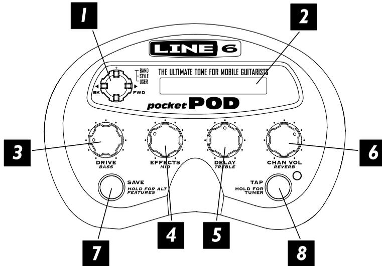
**1 4-way Navigation Button** – This button is your gateway to many of the fabulous features in your Pocket POD. By pressing on the top, bottom, and sides of the button, you'll be able to navigate **Up**, **Down**, **Left**, and **Right** to access the following functions:
