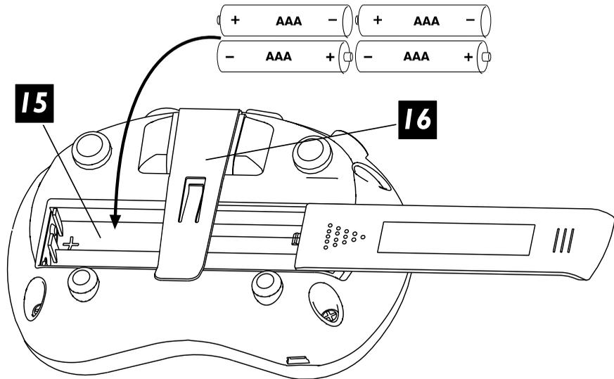
**15 Battery Compartment** – Pocket POD can run off (4) AAA batteries. To install them, slide off the battery door, insert the batteries in the orientation shown, then slide the battery door back on. Make sure you only use non-rechargeable alkaline batteries and dispose of them properly when they run out of juice.
