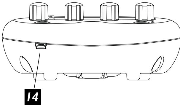
**14 USB** – You can connect Pocket POD to your Macintosh or Windows computer via the included USB cable and it'll automatically show up as a MIDI device. No drivers are needed!
