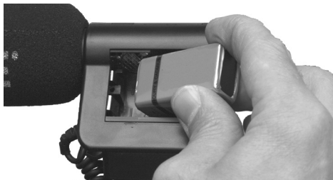
Figure 3 - Inserting the battery
