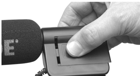
Figure 1 - Sliding open the battery cover
