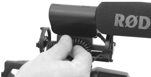
Figure 6 - Correctly mounting the cable
