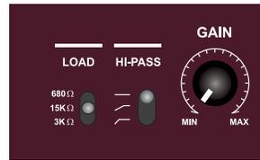
Set the GAIN to the MIN position, set the 3-position LOAD switch to the middle 15k position and the 3-position HI-PASS switch to the top 'flat' position. This is a good place to start before experimenting with the switches.
